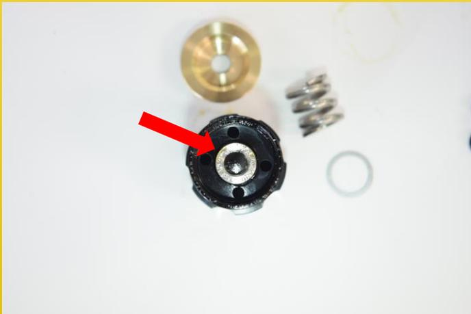
After separating the two you will be able to work the spacer off. Removing the reg seat, indicated in photo, will be the next step.
