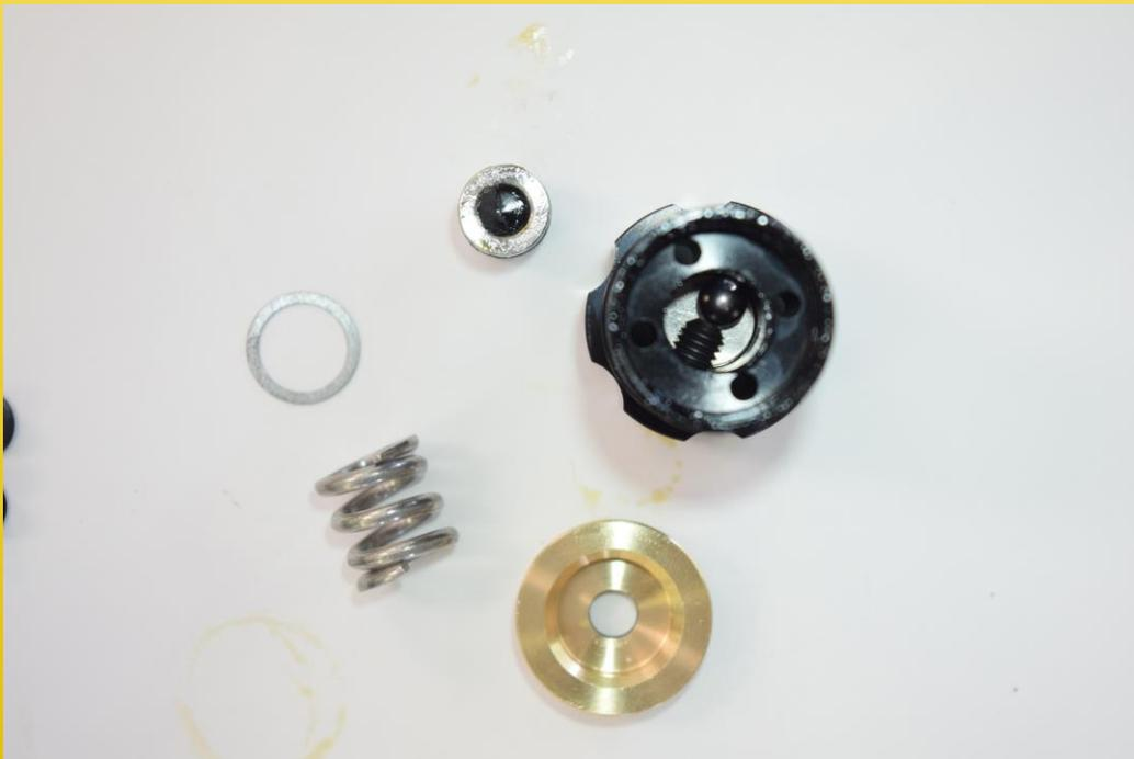
After setting the reg seat out you will see the adjustment screw, ball bearing, and base plate. You shouldn't need to take these out but just in case you will find instructions below.
