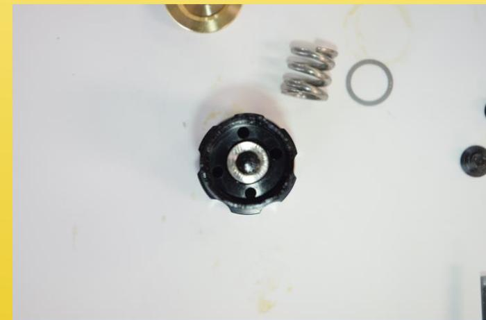
Be sure the seat is pressed all the way down and meshes with the bearing and screw before continuing assembly.
