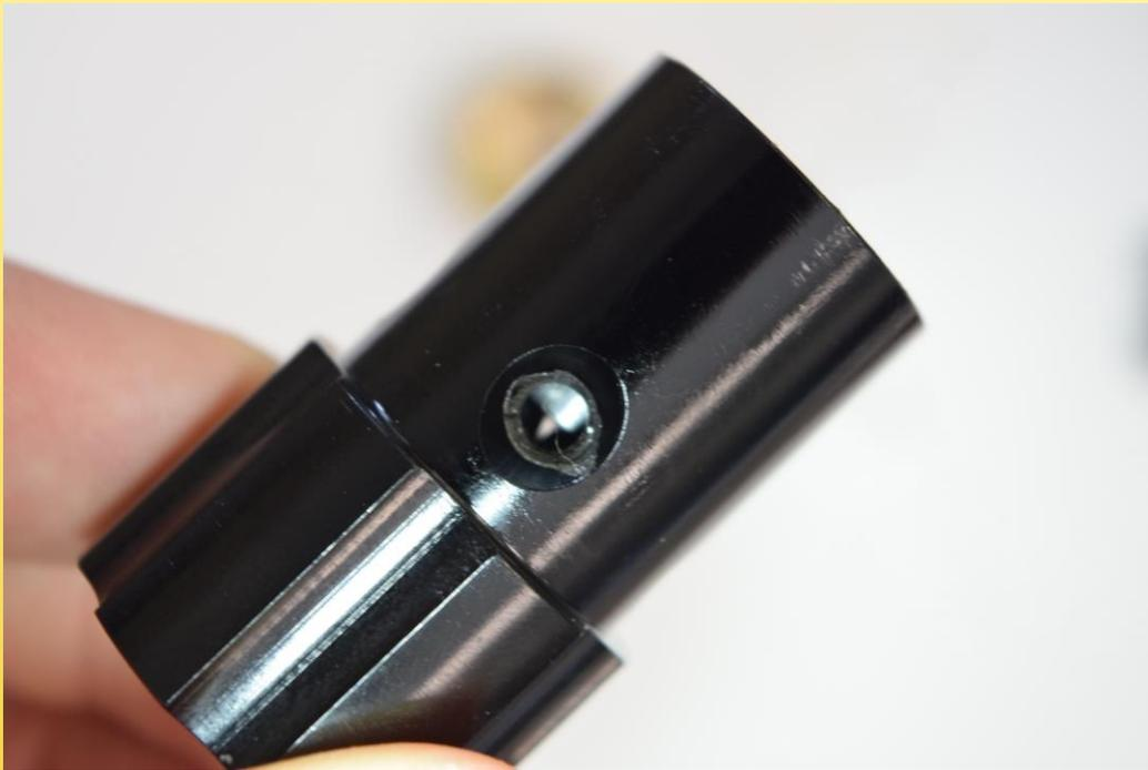
It is easiest to remove the reg seat by sliding a thin object into the side of the reg base through one of the set screw holes. You can then push up on the seat and slide it out of the base.
