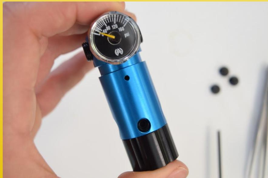
Be sure the adjustment screw lines up below the gauge for proper placement and put in the three set screws.
