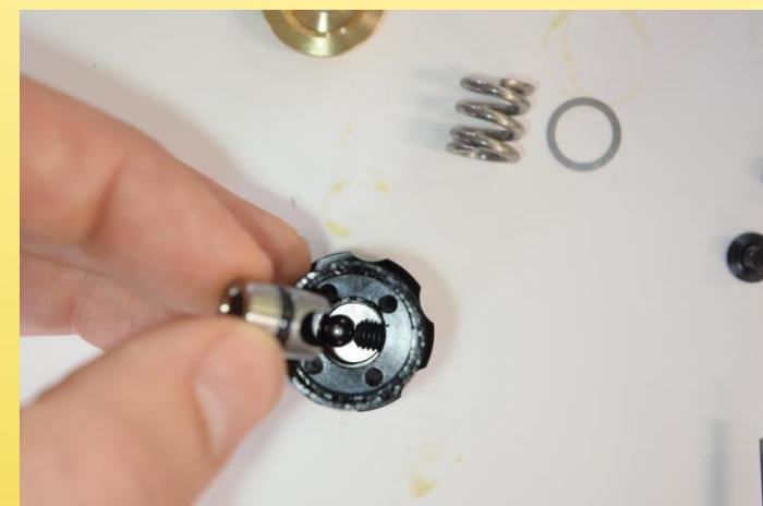
Next insert the reg seat into the reg base. Be sure the seat is properly oriented to the screw or you will not be able to adjust the pressure. The channel in the seat should open towards the screw.
