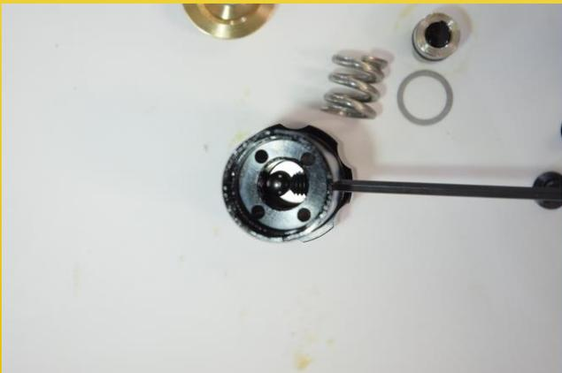
To properly install the adjustment screw you need to secure the bearing with the screw. Tipping the reg base so that the screw falls to the side opposite the adjustment screw hole will keep the bearing in place while you install the screw. The screw should securely hold the bearing in place.
