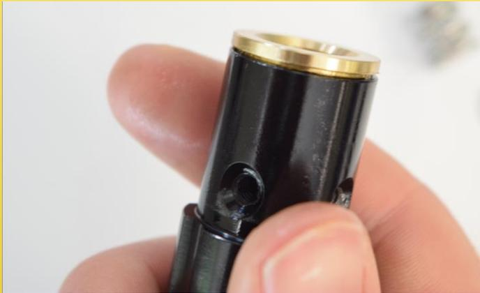
You will need to separate the spacer from the base by sliding a thin object between the two. Typically your thumbnail will work.
