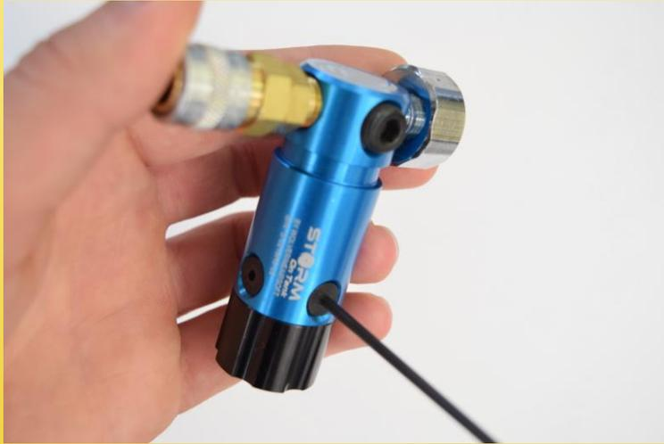
Begin by removing the three set screws from the regulator with a 3/32 in Allen Wrench. Be sure the adjustment screw is completely threaded into the regulator.
