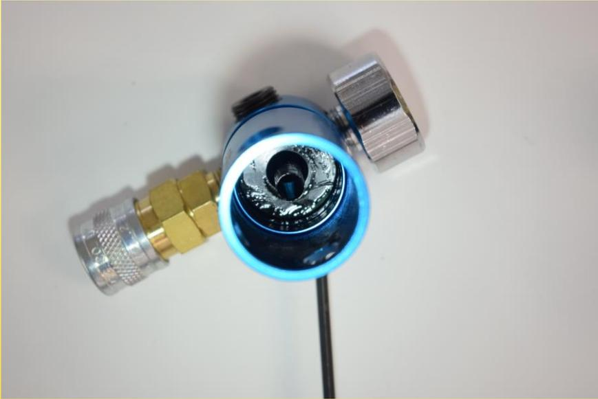
Next, remove the piston from the regulator cap.
