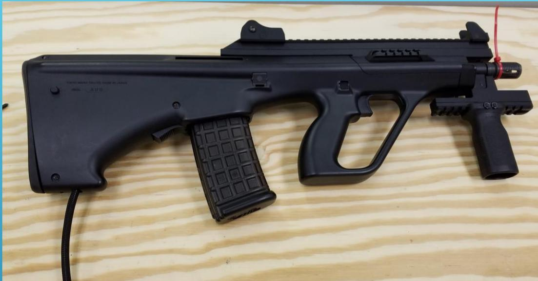
To route the air line, we simply drilled a hole in the lowest point on the stock. We found it easier to install the gearbox if we put an extended air line on the unit; this allows you to feed in the air line before sliding the gearbox into the body.
