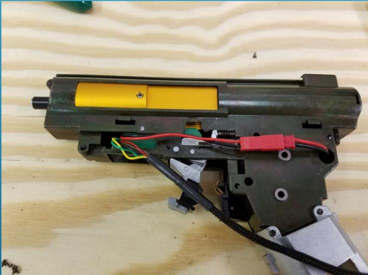
To activate full auto with the two stage trigger it was necessary to attach two leads to the connectors on the selector switch as seen in the first photo. These wires were then fed around and through the gearbox and soldered to the pads to complete the circuit. You can see we installed a plug between the two solder points to make disassembly of the gearbox easier.
